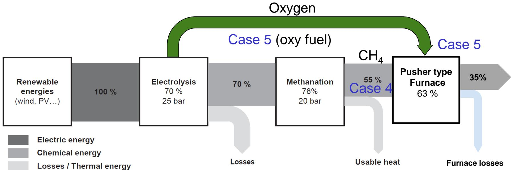
$$\eta_{\text{electrolysis}} = 0,70 \frac{\text{kWh}_{\text{H}_2}}{\text{kWh}_{\text{el}}}$$
